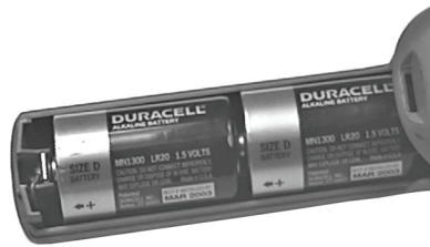
Figure 1: Properly Installed Alkaline Batteries
