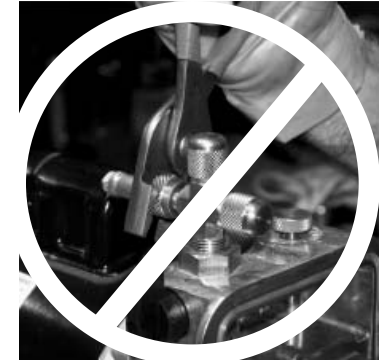
Figure 15 DO NOT WRENCH DOWN COUPLER
