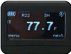
Saturation temperature for selected refrigerant at the given pressure
