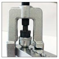
Step 2: Slide the flaring cone over the tube as shown.
