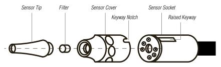
To install sensor cover: align notch with raised keyway and insert straight on (do not twist) To remove sensor cover: pull straight out (do not twist)
