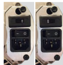
Sliding switch for 115v or 230v
